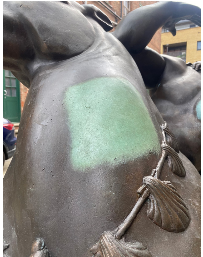
EARLY TESTING ON SEA PIECE AT RUPERT HARRIS CONSERVATION'S STUDIO IN LONDON TO FINALISE ITS RESTORED PATINA
